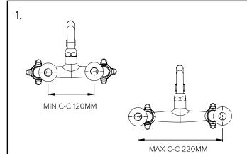
The sink faucet can be installed with centres that are between 120mm and 220mm
