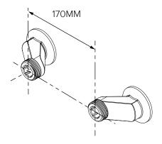
Install the adjustable 15mm offsets making sure that they are level and aligned with the faucet body
